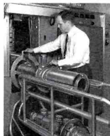
With this unique carriage, klystron change can be accomplished quickly.
